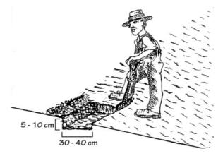
iv. Place large stones along the base of the trench and on the down-slope side to create an "anchor line."
