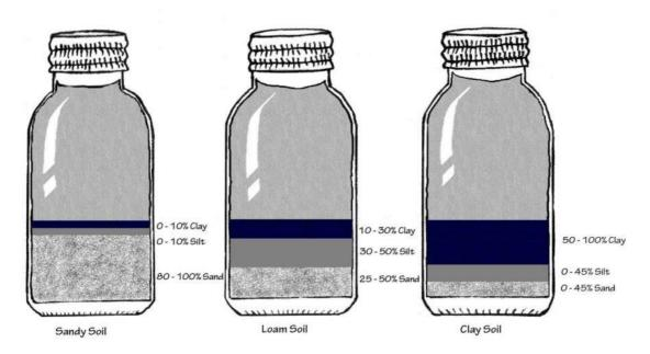
Figure 5.6: Using the bottle test to estimate the proportion of soil separates in a sample
