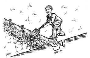
Dig a shallow furrow along each contour line (30 - 40 cm deep and 50 cm wide) and place the soil on the down-slope side of the furrow.
