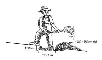
iii. Dig out a shallow furrow (about 50 cm wide and 30 cm deep) along each contour and place the soil on the down-slope side of the furrow to create a ridge (about 20-30 cm high).
