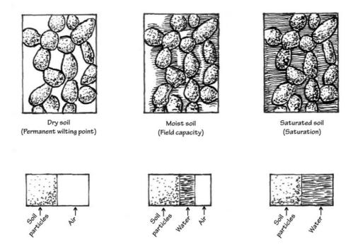
Figure 5.4: Amount of water and air in dry soil, moist soil and saturated soil
