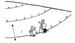
ii. Mark out the contour lines on the slope, three meters apart.
