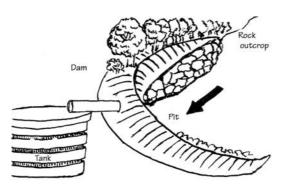
Figure 1.5: Water overflow is directed into a storage tank
