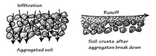
Figure 5.8: Infiltration vs Runoff (From: WHC Manual, WRC, 2010)
