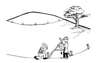
Mark out each contour line using an A-frame or line level. If necessary, make slight adjustments to the position of the pegs so that the lines form a smooth curve.
