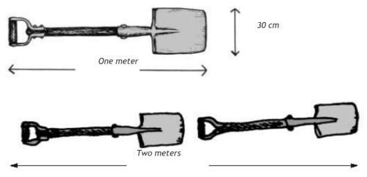
Figure 5.15: Easy measurements using a spade
