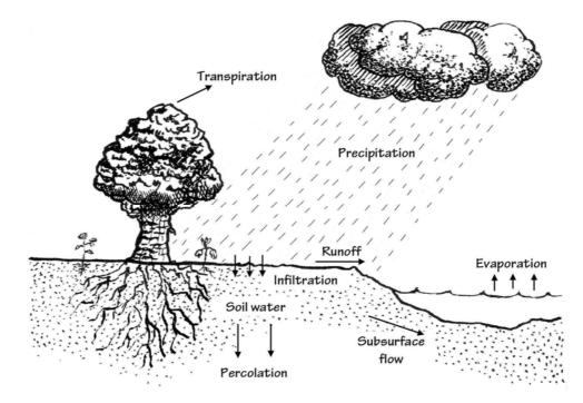
Figure 5.1: Water movement through the soil
