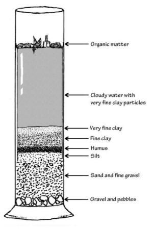
Figure 5.5: Bottle test showing proportion of soil separates (From: WHC Manual, WRC, 2010).
