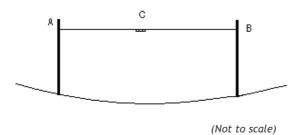
Start at the edge of the field. Person A holds their pole in a vertical position and stands still, while person B moves up and/or down the slope until the line level, which is read by person C, gives a level reading. Points A and B are then marked with pegs.
