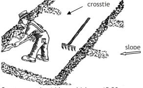
iv. Create crossties (ridges which are 15-20 cm high) every 3 meters. Ties must be lower than the main ridges so that water never flows over the ridges.
