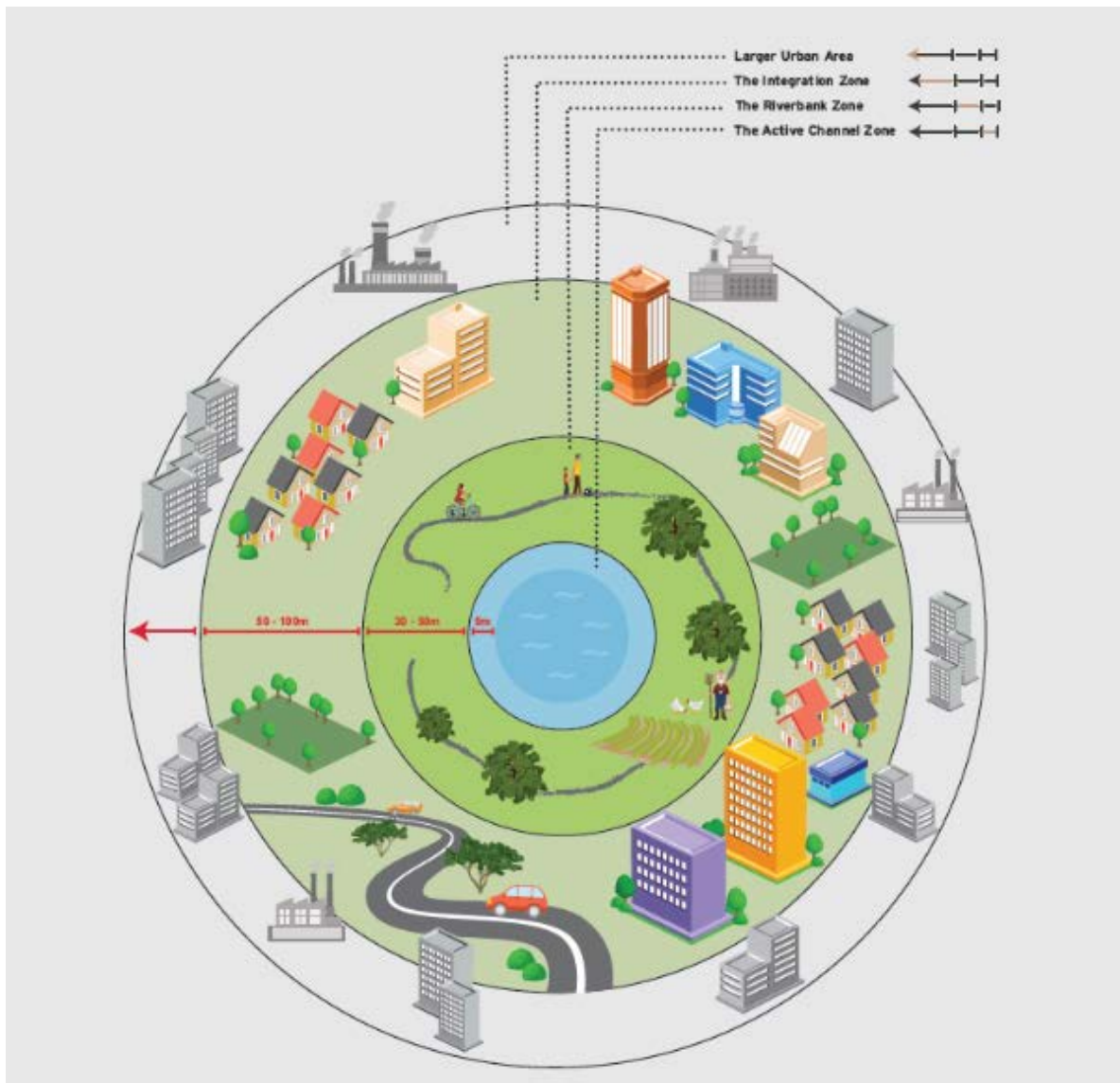
Figure 5b: Diagram illustrating different setback zones based on best practice (H. van den Berg and S. Braid, 2017)
